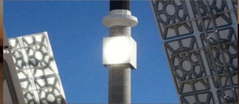
Highly accurate GSP measurement + sophisticated control software precisely centers beam on target
