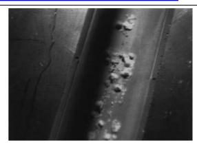
with pit corrosion damage on fuel plate cladding over fuel material region.
