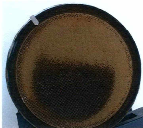
Figure 16c Photographs of an Average Restriction (21 inches of water @ 100 g/s) Canadian Vehicle Inlet Element Inlet Face
