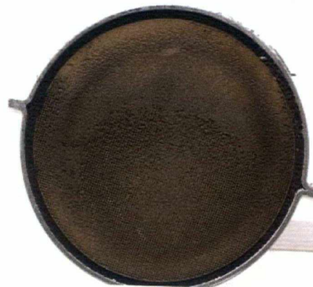
Figure 6 Picture of a catalyst sampled from the "Four Corners" area of the USA where MMT was sold in limited amounts
