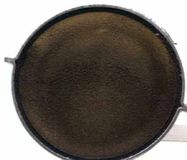
Figure 6 Picture of a catalyst sampled from the "Four Corners" area of the USA where MMT was sold in limited amounts
