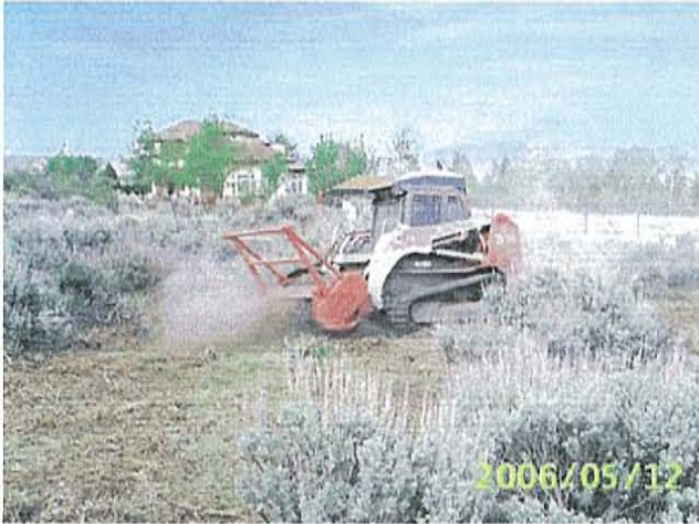
Above: Rubber-tracked vehicle with Fecon mastication power head at work in the Eagle Ridge Chapter. Below: Completed fuel break.
