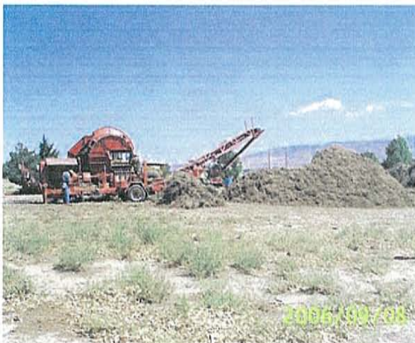
Above: Community biomass pile prior to being converted to ground chips for dust control mitigation. Below: A tub grinder converting raw biomass to ground chips. Approximately 100 tons of hazardous fuels were treated in ...
