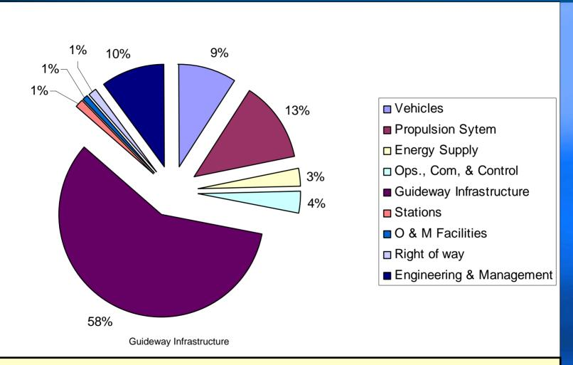
Total construction cost for Anaheim to Las Vegas: \$12.1B (2000\$); Guideway Infrastructure is large fraction of capital cost of High Speed Maglev
