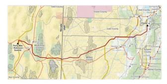
Transcanyon Cross-Tie Project: The BLM Fillmore (Utah) Field Office expects in April to publish a Notice of Intent in the Federal Register for a proposed transmission line connecting central Utah and east-central Nevada. The 1,500 MW, 500 kV HVAC line would be located within the existing Western Electric Coordinating Council-designated corridor or BLM utility corridors. It would
