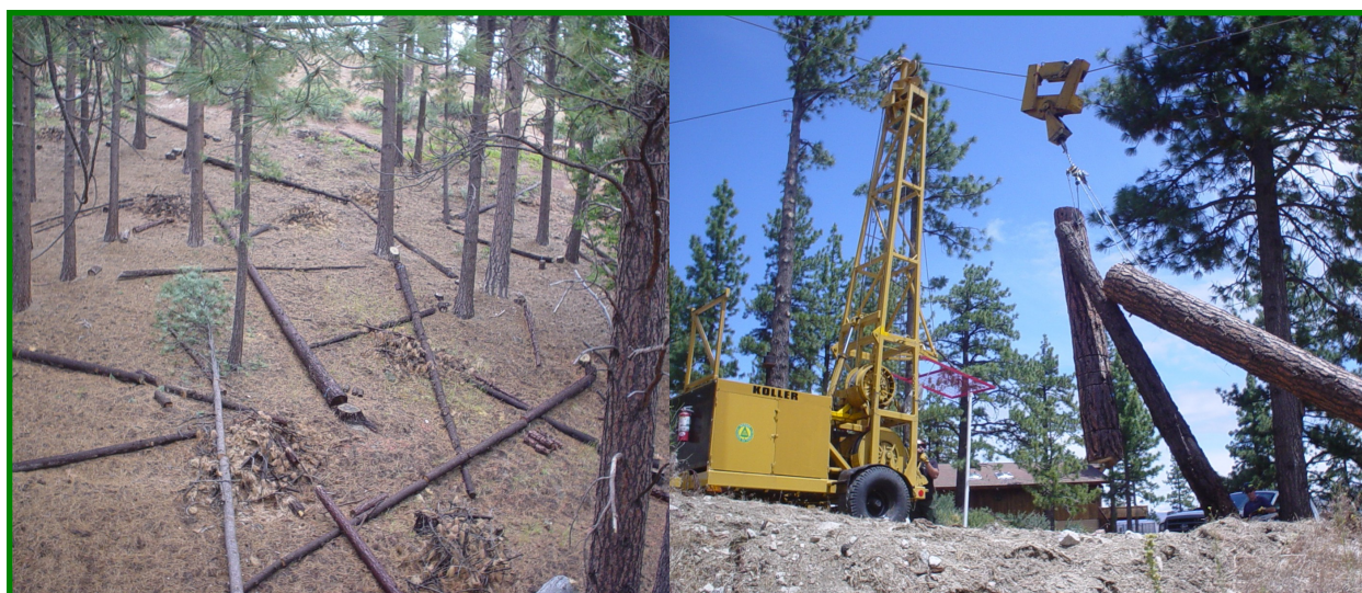
The NDF cable yarder allowed logs cut as part of a Forest Stewardship project to be efficiently and quickly harvested from an area with steep terrain.
