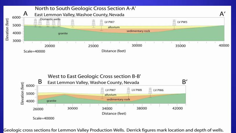
Lithology shows depth to granite, sedimentary rock and alluvium in East Lemmon Valley. Note the domestic wells
