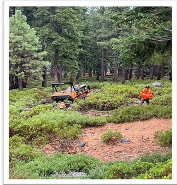
Low impact mastication technology being utilized by NLTFPD to reduce hazardous fuel loading in the forest.
