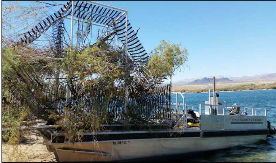
PVC structure stuffed with nonnative tamarisk that was cut down along the shore lines and ready for deployment on the habitat barge at Lake Mohave
