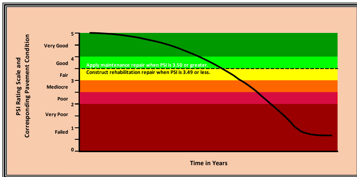
FIGURE 3. Timing for Repair Strategies Based on PSI Rating System
