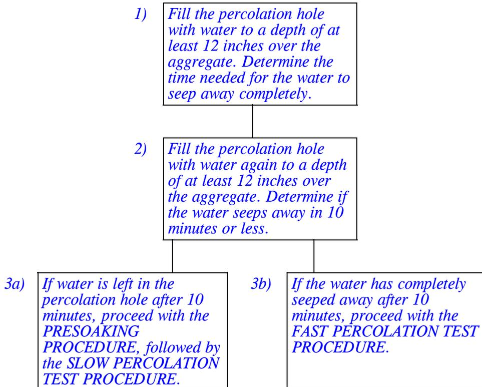
Sec. 41. *The following flow chart illustrates the fast percolation test procedure:*
